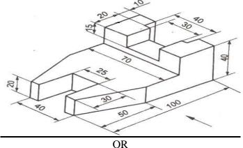
Draw its i) Front view ii) Top view and iii) side view of the object shown in figure. All Dimensions are in mm.
